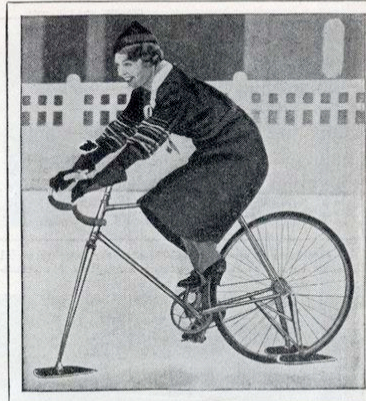
This ice-cycle, an ordinary bicycle fitted with steel runners, provides thrills of summer bicycling on ice during the winter. Dolly Davies, actress, tries out the French invention.
